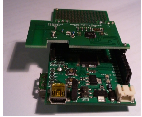
Figure 2: ZigFlea board mounted on top of the CUI32 board. The antenna is the part sticking out on the left side.
