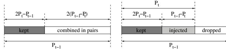
(a) Combining the last  $2(P_{t-1} - P_t)$  particles with lower weights (b)  $P_t$  new particles are formed
