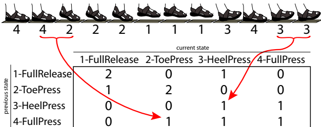
Figure 5: A simplified example of a short walking sequence made from 12 successive states. Below is the corresponding pheromone table .
