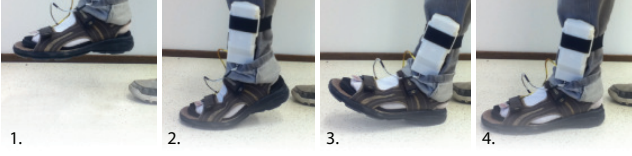
Figure 3: The data is quantised into four states: 1-FullRelease, 2-ToePress, 3-HeelPress, 4-FullPress
